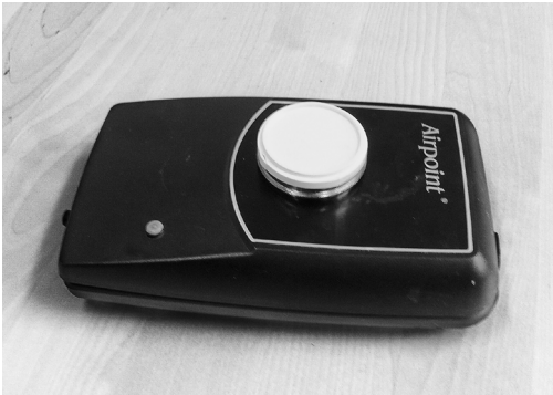
Figure 12. Virus air trap sampler designed to capture virus particles from the air.
