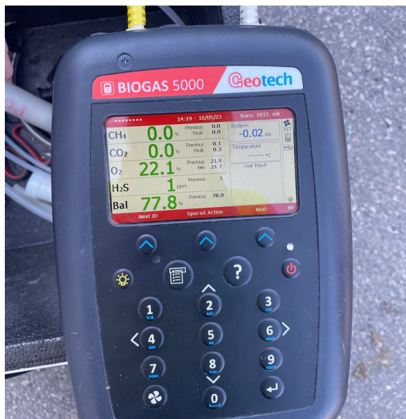
Figure 3. Data from the Geotech Biogas 5000, only CH 4 concentration is of interest.
