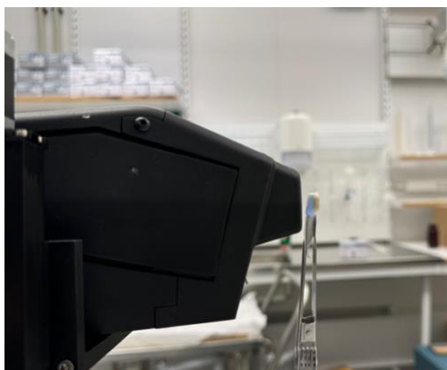
Figure 17. The swab was held aloft by a clamp, and the red detection focal point of the XRF test is aimed at the varnish residue on the swabs.
