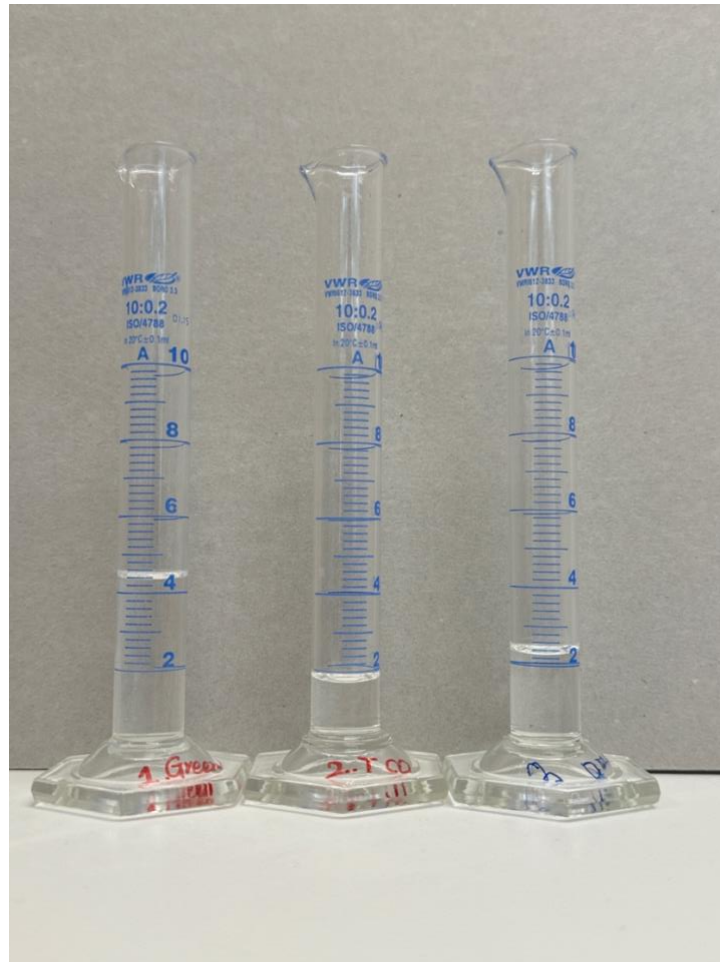
Figure 24. Remaining amounts of the three solvents after 13 days of evaporation, from left to right: GVR, TACO2, and DMSO blend.
