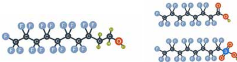
Figure 2.2: Display of the chemical structure of PFAS. Left: Polyfluoroalkyl substance with a partially fluorinated, hydrophobic chain and a hydrophilic functional group. Right: Two legacy perfluoroalkyl substances with each an eight-carbon fully fluorinated chain and a carboxylic acid (PFCA) as functional group of perfluorooctanoic acid (PFOA; top) and a sulfonic acid functional group (PFSAs) of perfluorooctanesulfonic acid (PFOS; bottom). PFCAs will be color-coded brown with darker colors for increasing chain length, while PFSAs will be color-coded blue with similarly darker colors for increasing chain length throughout the thesis and papers.
