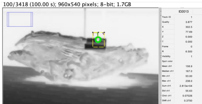
Figure 5. A FIJI plugin called Trackmate was used to measure shell gape over time by tracking the position of a dot on a marker glued to the top valve of the oyster.
