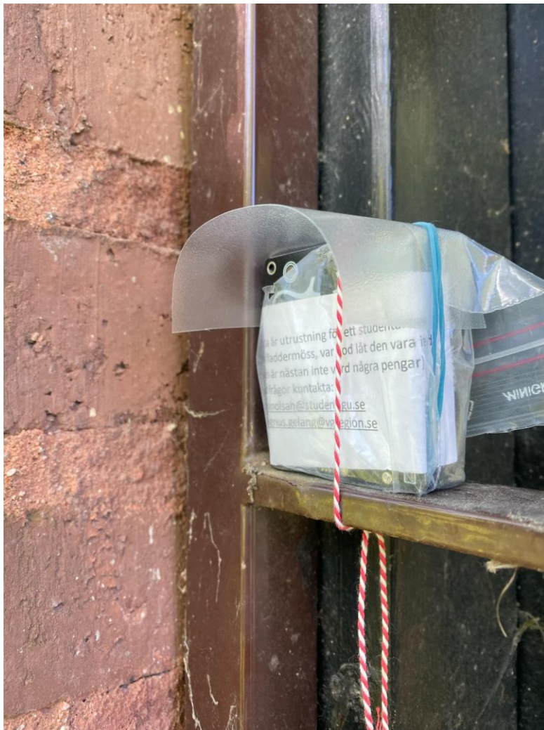
Figure 2: One of the bat detectors set up at its designated recording site, protected from moisture and other disturbances by a plastic bag and cover. Photograph by Magnus Gelang.
