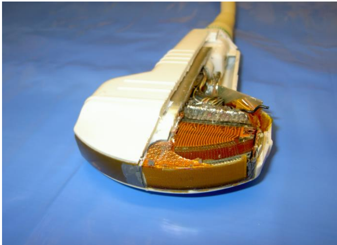
Figure 2. A curved linear array transducer with the housing sawn apart. Photograph by Benny Stenborg (reproduced with permission).
