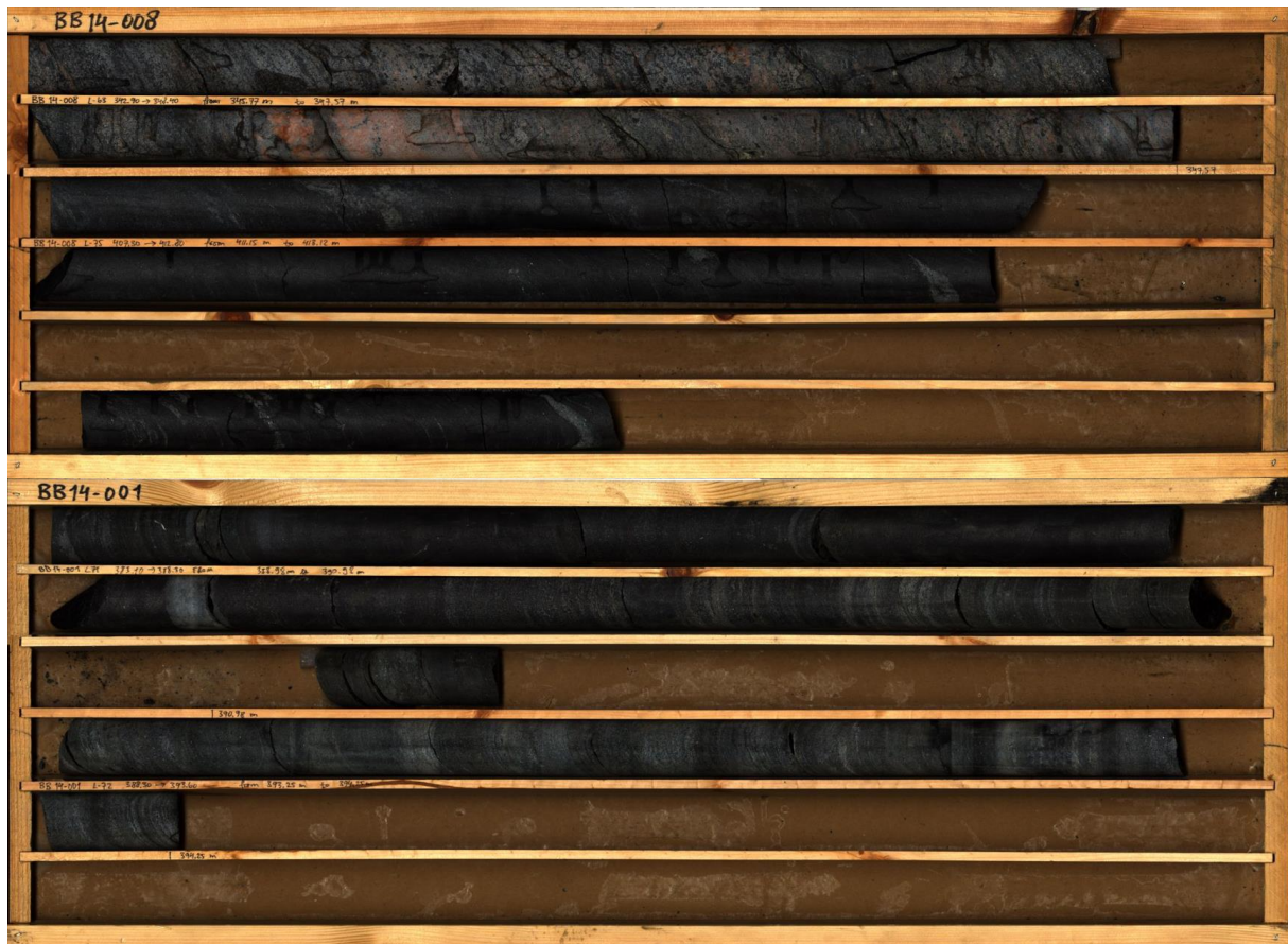
Figure 4. Drill core images created by the Minalyzer CS.
