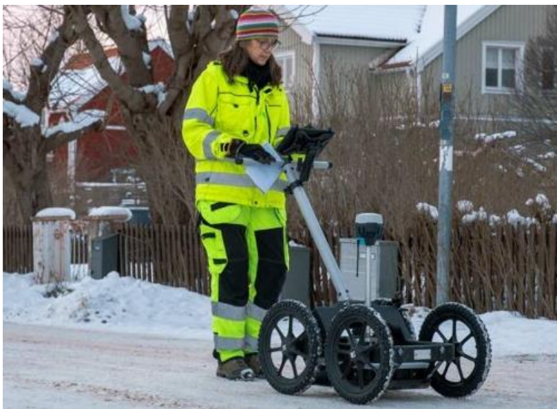
Figure 4. Picture describing a GPR in operation. From Guideline Geo AB (n.d.).
