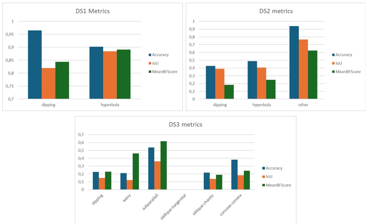
Figure 24. Metrics for each class in the datasets DS1, DS2, and DS3. The graphs show the accuracy, the IoU, and the mean BF score. In general, the results of DS1 show the highest values and the lowest spread among the classes.
