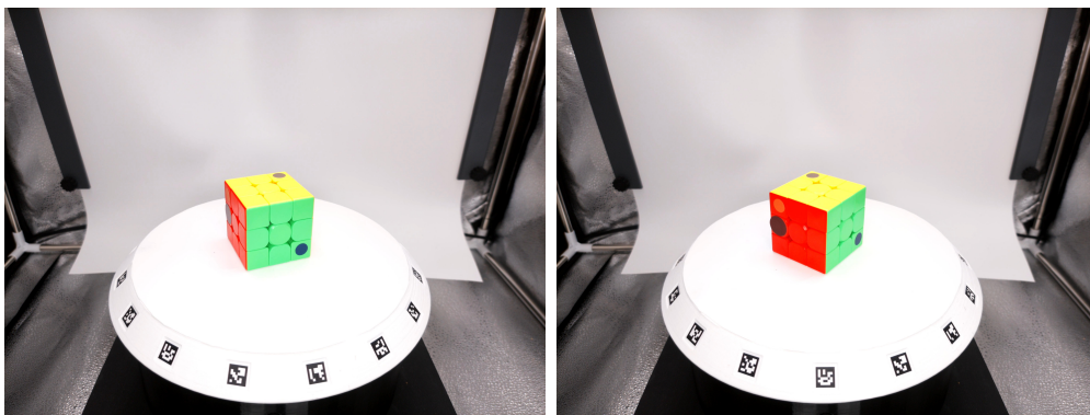
Figure 3.1: Two frames in a 30-degree angle from the generated dataset used in our study. The cube has stickers on different sides marking the areas of interest which the models track.
