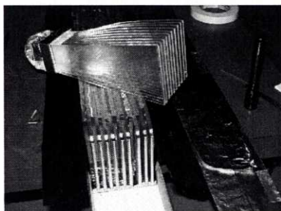
Figure 3.8: A photograph showing a disassembled paddle of LAND. The altering sandwich structure of the plastic scintillator and iron converter is clearly seen.
