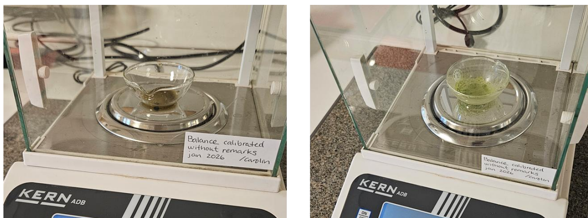
Figure 11. Gravimetric dry-weight determination of fresh biomass. Left: pre-weighed crucible containing a 1 ml aliquot of freshly harvested Craspedostauros sp. biomass suspension prior to drying. Right: the same crucible after microwave drying at 500 W for 1 min to constant mass.
