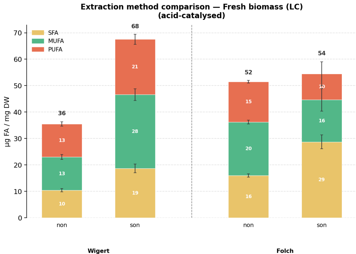
Figure 16. Total FA and FA class composition for untreated control (non) and probe ultrasonicated (son) fresh biomass (LC) extracted with Wigert vs Folch (acid-catalysed, mean \pm SE, n = 3 except the Folch LC_son_0d where n = 2 ). Hatched bars indicate standard error.
