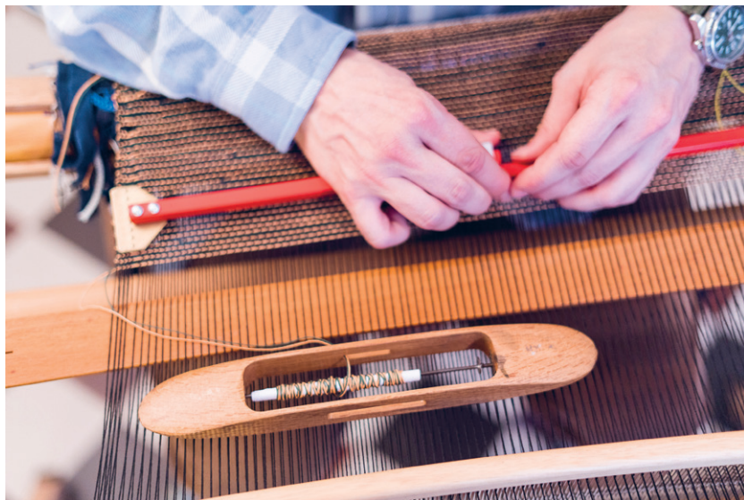
Figure 4.41 Kalalanka 6-ply cotton thread used for the warp in the Weaving Kiosk at Collaboratorio (Sep. 2017). The loom was threaded with four threads per centimeter and a weaving width of 40cm. Photo: Jukka Kiistala.
