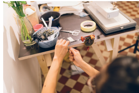
Figure 4.14 Bobbin winder attached on table and in use in the Weaving Kiosk (Sep. 2018). Photo: Johannes Romppanen.
