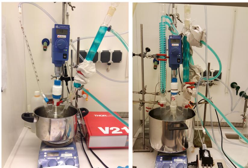
Figure 3.5: Synthesis set up for the 100 ml (left) and the 1000 ml (right) protocol.
