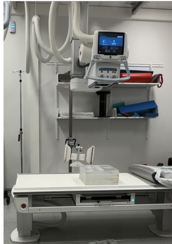
Figure 3.1: Photograph of the set-up for the measurements at Sahlgrenska University Hospital. The X-ray tube is located at the top, and the PMMA is placed on the patient table below. Under the table, the anti-scatter grid, AEC, and detector is located.
