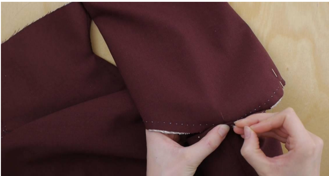
Figure 22. I decided it would be easier to sew in the sleeves before finishing the lining. First the seam allowance of the outer fabrics armhole was folded in and pressed and I also cut into the seam allowance to allow it to lay smooth on the inside. I then pinned in the sleeve, placing the folded edge of the armhole just past the prick stitch around the sleeve, matching up the seams to the placement of the sleeve. This was then sewn with prick stitches in dark red silk thread, 1mm long and 3mm apart through the two sleeve layers and the outer fabric of the bodice.
