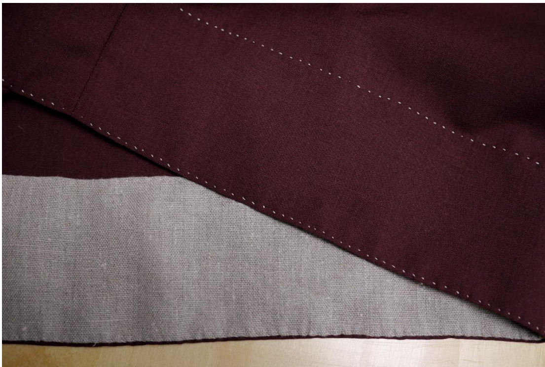
Figure 4. I folded and pressed the hem of the wool fabric and the edges of the hem facing in linen. The facing was sewn with hem stitches around 1mm long and 4mm apart. The top of the facing was sewn down with running stitches 1mm long and 4mm apart.
