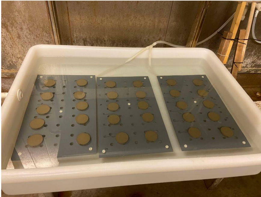
Figure 7. The mesocosm experiment. A total of 30 sediment cores submerged in seawater connected to a flow-through system from the Gullmar fjord. The mesocosm was covered by a blanket and was left there for 30 days. The temperature was set to 10 °C.
