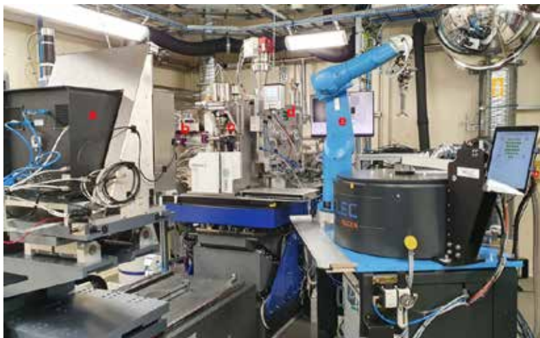
Figure 1.8: BioMAX experimental hutch: a) EIGER 16M detector, b) REX with HClab and cryo-jet, c) Arinax MD3 microdiffractometer, d) BCU, e) ISARA sample changer.
