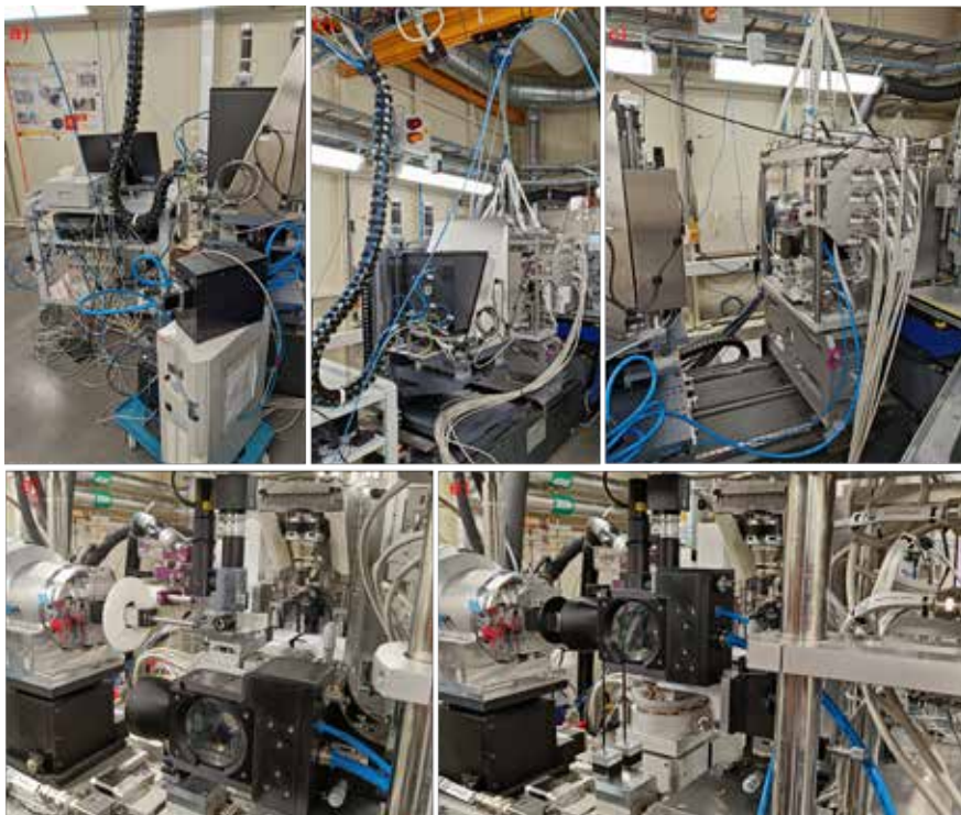
Figure 4.13: Roadrunner II at BioMAX; a) control computer and humidifier, b) back view after installation, c) side view, d) sample position before humidity chamber, e) sample position with humidity chamber
