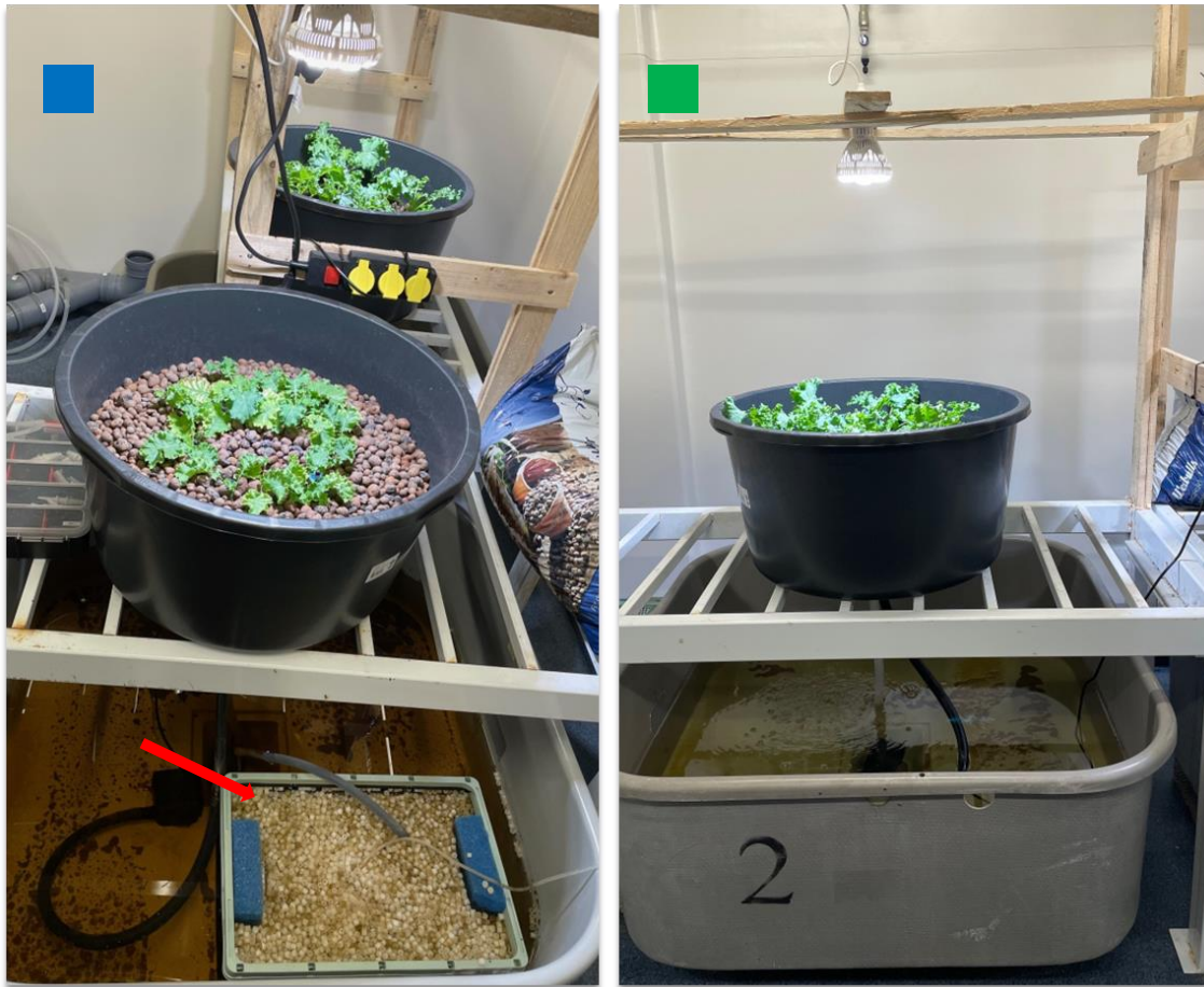
Figure 6: Experimental setup, left: aquaponic treatment (red arrow=biofilter), right: fertilised treatment without biofilter
