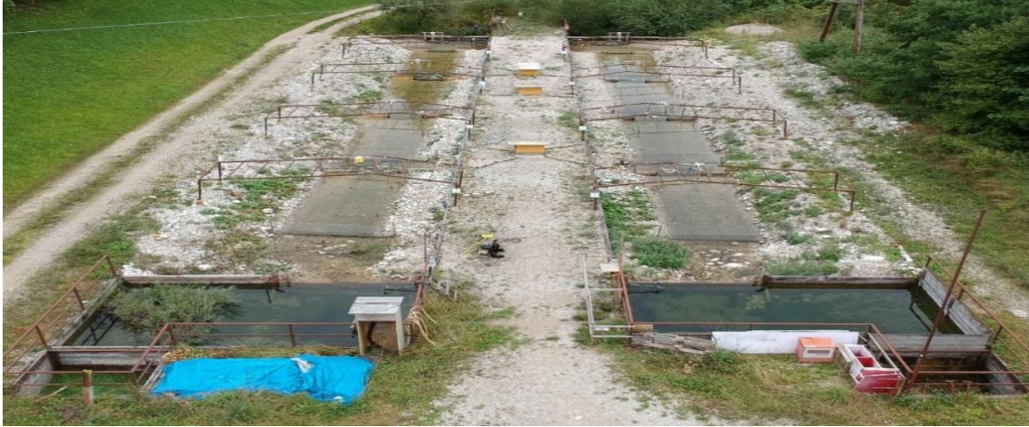
Figure 2. Hitec Flume with 8 sections divided into two artificial streams located in Lunz am see, Austria. Photo: Libor Závorka
