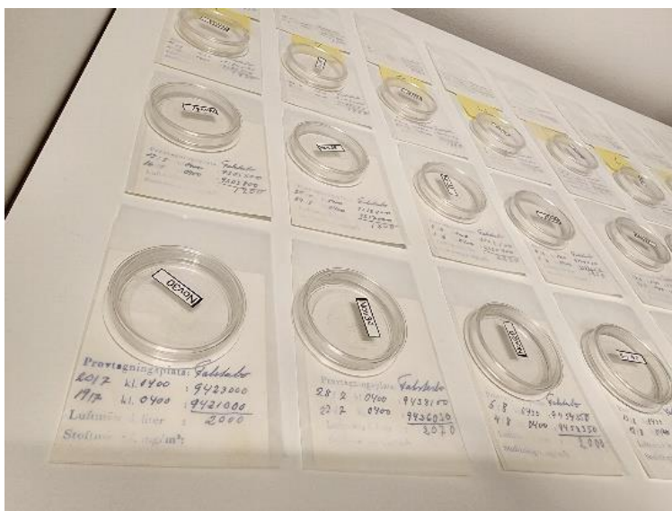
Figure 3.3: Filters cut and placed in petri dish.
