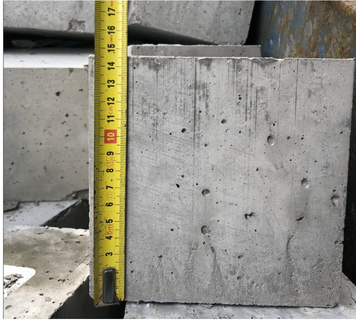
Figure 6: The sizes of the concrete cubes vary. This affects the compressive strength measurements which depend on the surface area.
