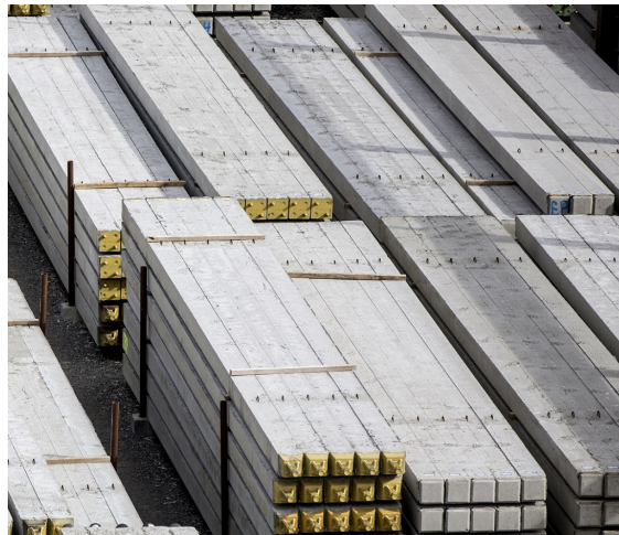
Figure 1: Concrete piles in storage [1].
