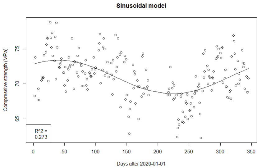
Figure 23: Sinusoidal model fitted to compressive strength over time for 2020.
