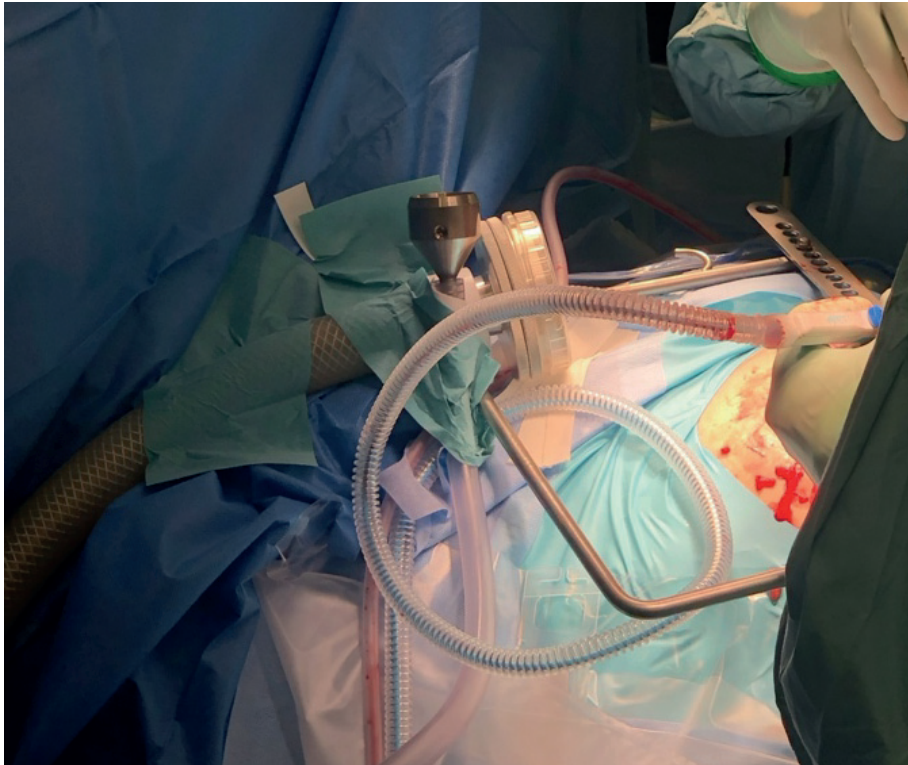
Figure 12. Placement of the mouthpiece of the Sartorius MD8 (horizontally) and the iso-kinetic probe of the BioTrak 9510 BD (vertically). The photo is taken by Frans Stålfelt, with the permission to use by Karin Löwhagen. Figure found in Stålfelt F, Caous J, Svensson Malchau K, Björn C, Mohaddes M. Evaluation of real-time biofluorescent particle counters for monitoring airborne contamination in orthopaedic implant surgery compared to conventional air sampling Antimicrobial Stewardship & Healthcare Epidemiology , 2025;5(1): e93
