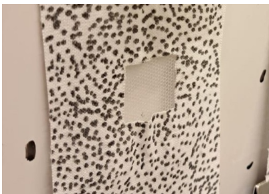
Figure 31. Adhesion failure in the adhesive nylon net sample (batch 3) after 100hr on the fixed-load test
