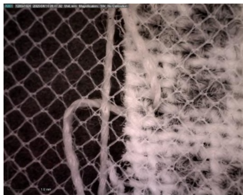
Figure 37. Stitch needle hole of stitched polyester tulle sample (batch 2), after fixed-load test, bigger needle hole
