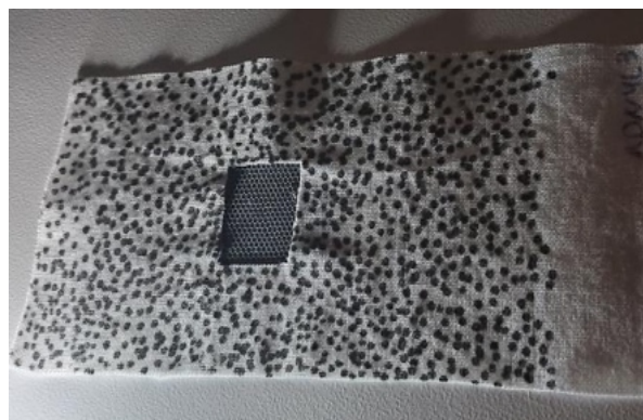
Figure 32. Deformation in the adhesive nylon net sample (batch 3) after 167hr on the fixed-load test
