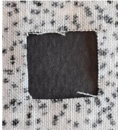
Figure 82. Untreated control sample after fixed-load test, back face
