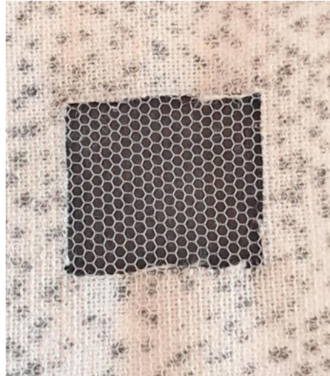
Figure 98. Nylon net adhesive sample after fixed-load test, back face
