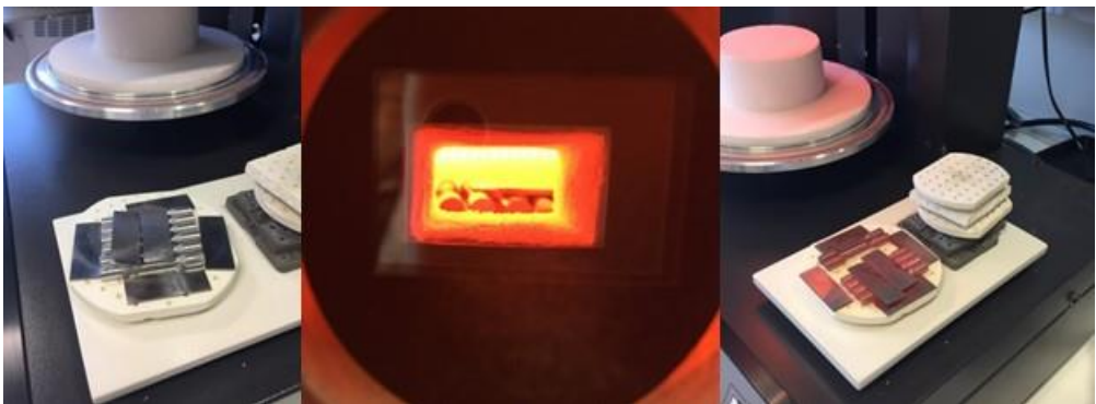
Figure 8. The firing of the specimens. After each firing process ( n= four), the specimens were left to cool down at room temperature.
