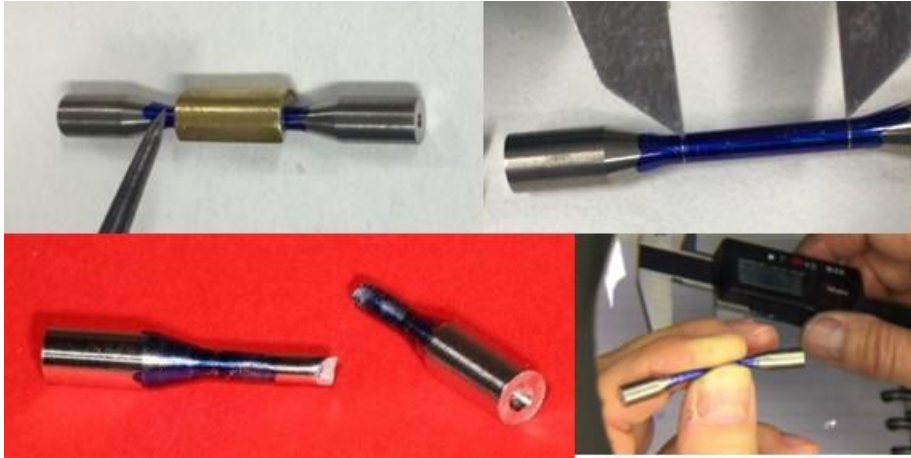
Figure 16. The manual measurement of gauge length before and after specimens' fracture. The gauge area was coloured with a marker, and two positions were curved with a pointy tip and measured before the test (upper). After the test specimens fractured, the two pieces were put together, and a re-measurement of the gauge length was done (down).
