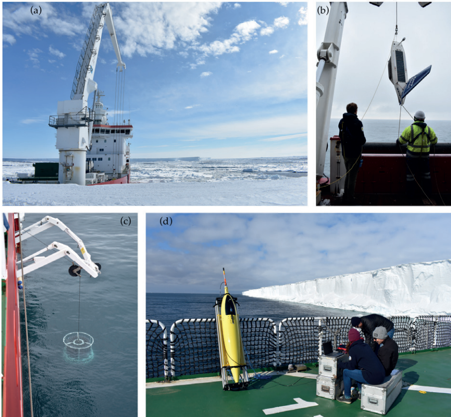
Figure 7.1: Images from the SO-CHIC 2022 expedition: (a) The S.A. Agulhas II moored alongside Penguin Bukta ice shelf, (b) Sailbuoy deployment, (c) CTD cast, (d) on-board Seaglider tests.
