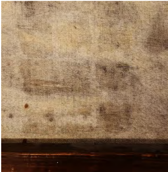
Figure 14. Paintings backside, closeup on backside of Evolon cleaning tests. Image contrast has been enhanced to increase the visibility of solvent migration marks.
