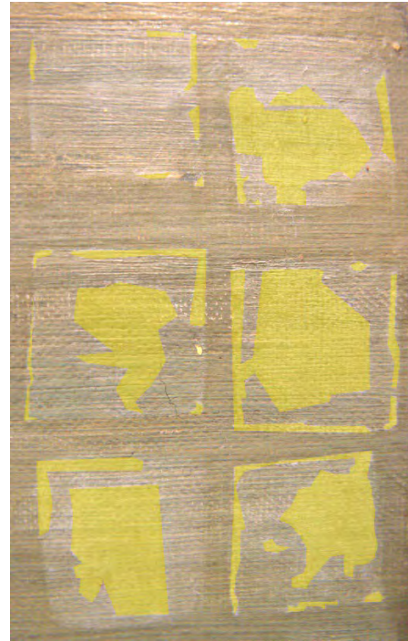
Figure 19. Close up to test patches of agar soaked in ethanol cleaning test, blanching marked in yellow.
