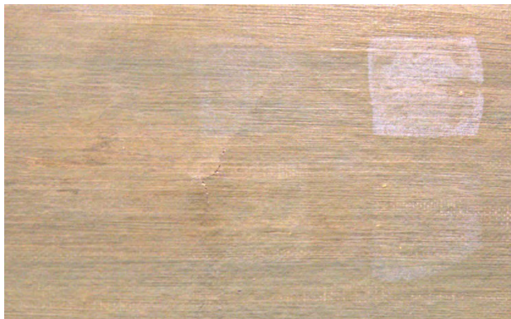
Figure 16. Close up to test patches of agar mixed with ethanol cleaning test.
