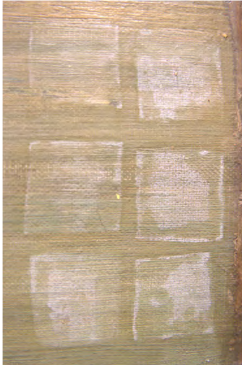
Figure 18. Close up to test patches of agar soaked in ethanol cleaning test.
