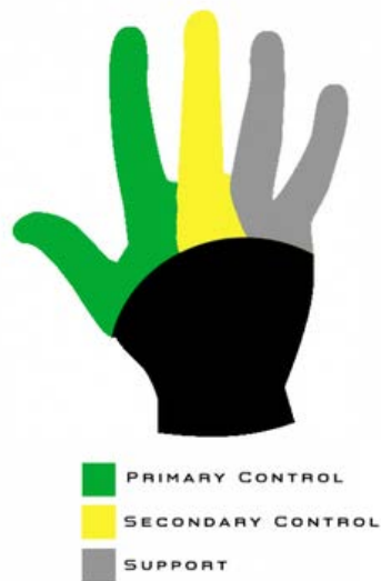
Figure 3.5: Three main “finger groups” that we need to keep in mind during controls design [10]
