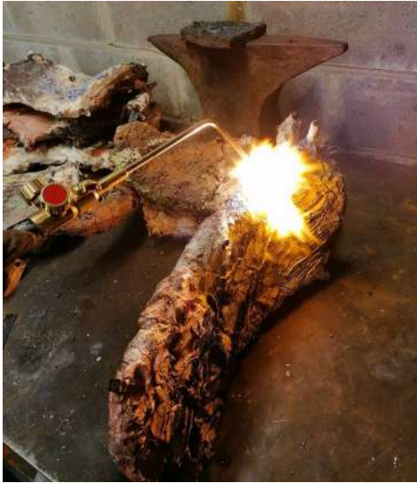
Vitrification of clay with a torch.
