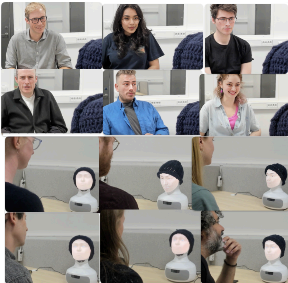
Figure 5.2: Session in progress. Experiment setting showing cameras placed behind the users and Furhat during the interaction. Images to the left show various positioning of gaze movements of the robot in accordance with the conversation flow (consent has been provided by the participants to use the images from the experiment for publishing purposes with faces being swapped/anonymized)
