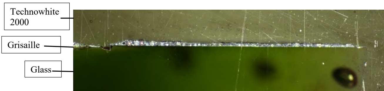
Figure 83. Microscope image of the cross section. The scale bar seen to the right is 50 μm. Photo: Eisfeldt, 2022
