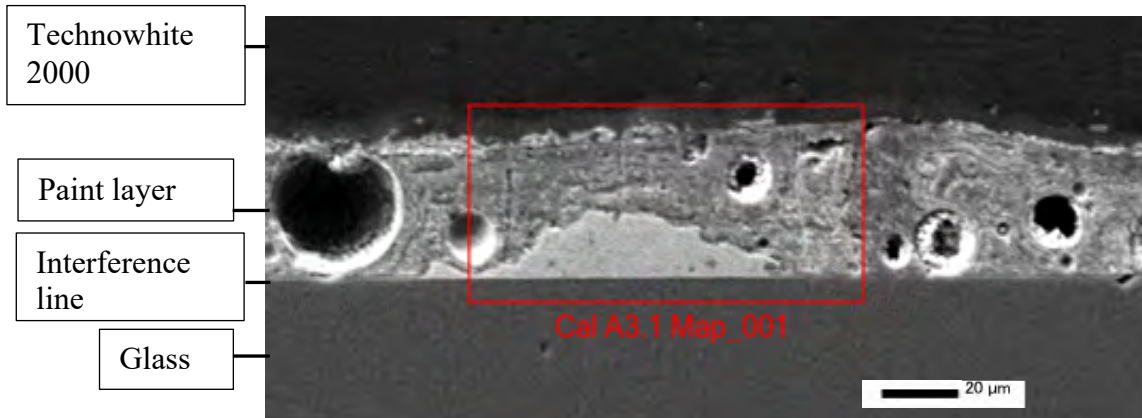
Figure 96. Image of SEM-EDS map 001 of the cross section of glass A. magnification x550. The scale bar is 20 μm. Image: Eisfeldt, 2022
