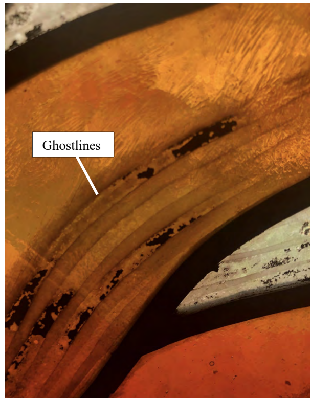
Figure 64. Paint loss and ghostlines of Callmänder's window in Varberg's church. Photo: Eisfeldt, 2022
