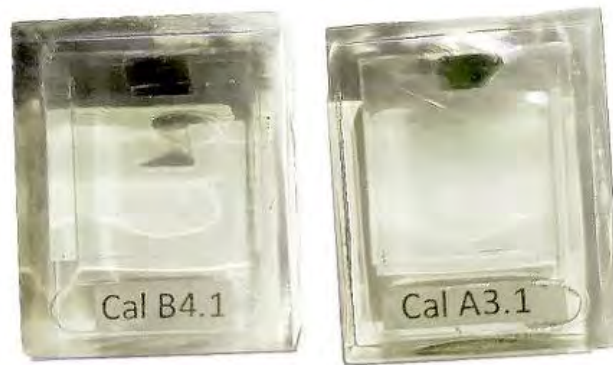
Figure 78. The two samples for cross section embedded in technowhite 2000. Photo: Eisfeldt, 2022
