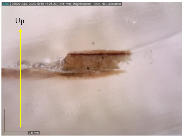
Figure 39. Cross-section from NMI 232, picture taken in regular light at 150x using a DinoLite.
