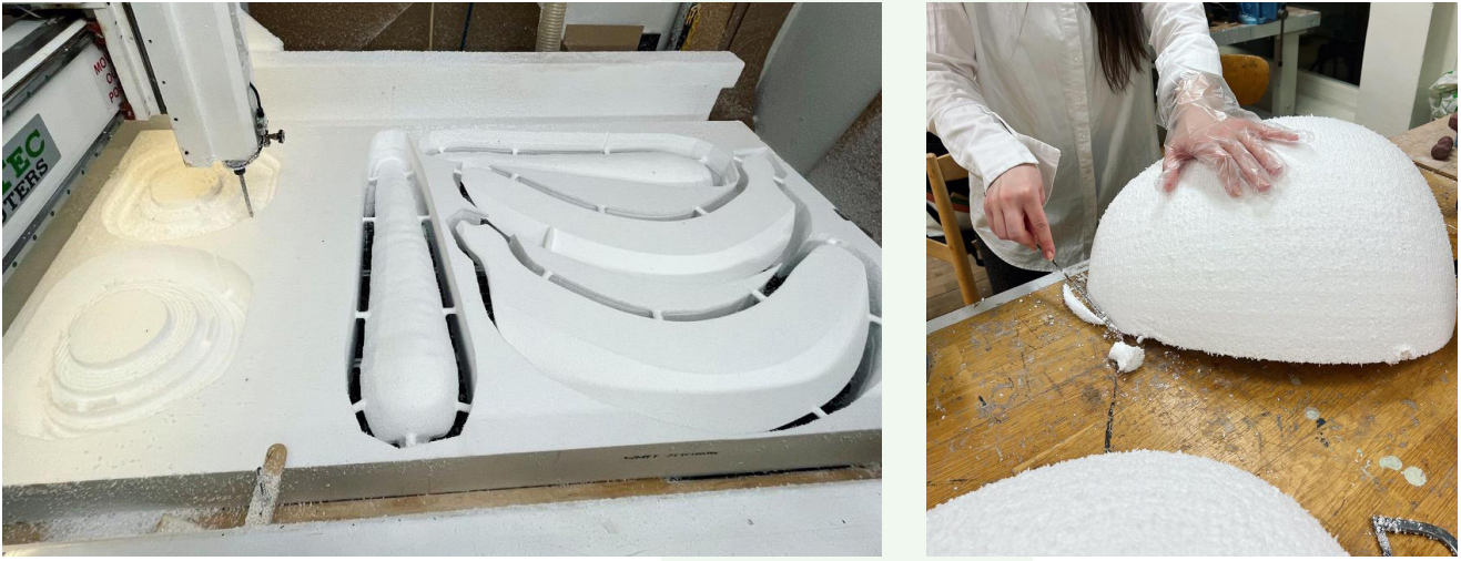
Fig. 4. CNC Milling and styrofoam shaping
