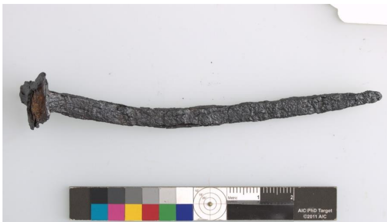
Figure 3: Specimen nr. 230 after mechanical cleaning.
