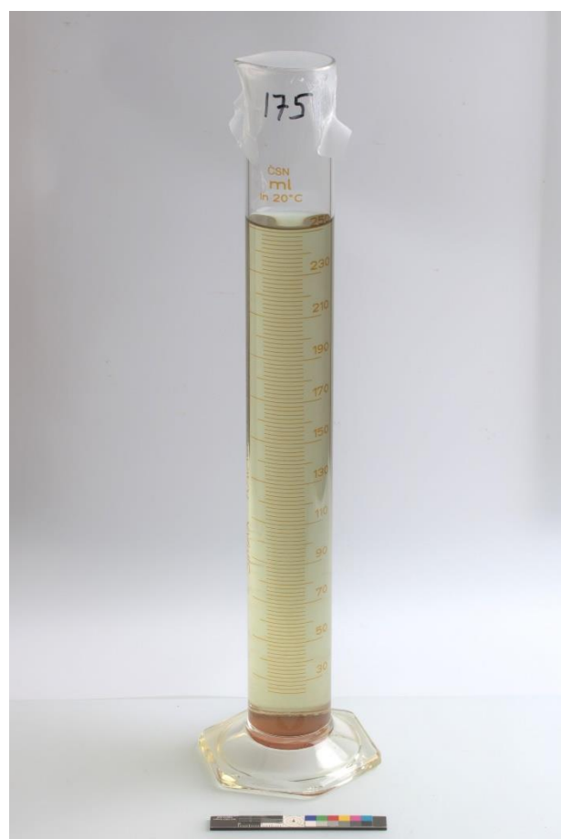
Figure 9: a residual chloride sample ready for analysis. Notice the green colour, and the layer of rust-brown precipitate at the bottom of the measuring glass, formed after filtration.
