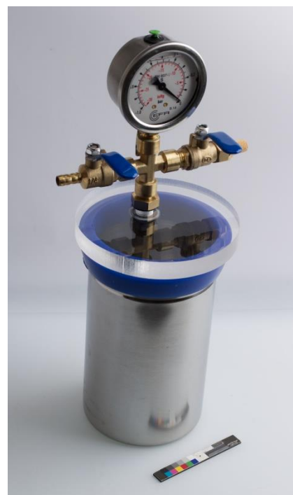
Figure 5: Stainless-steel vacuum containers by VacuumChambers.eu (VC0918SS) with manual valves, pressure gauges, silicone gaskets and custom-fitted acrylic lids were used in the study.
