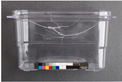
Figure 6: Stress-corrosion-cracking caused by pressure and contact with an alkaline solution on a polycarbonate FoodSaver® FFC002 vacuum container.
