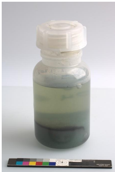
Figure 8: A specimen fully digested in sulphuric acid. Notice the bluish-green colour, the dark undigested material, and the layer of crystalline ferrous sulphate at the bottom of the LDPE bottle.
