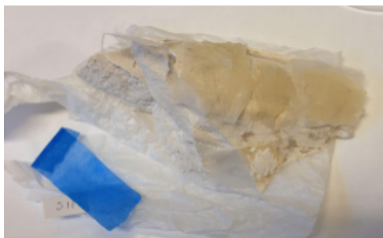
Fig. 22 - Preliminary tests for xanthan and Arbocel® systems on fragment S11.
