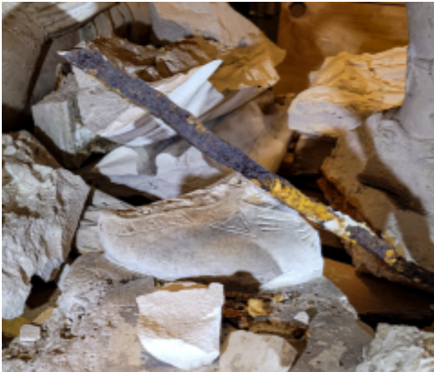
Fig. 6 - Deformed armature protruding from one of the sculpture's feet as well as parts of the fractured base. Stockholm Stadsmuseum. SSM 31130.
