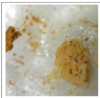
Fig. 38 - Cleaning sample, fragment B3. 3,5% Xanthan w. 2% EDTA, 5oz, 1h. Plaster particles stuck to the gel. Magnification: 67x.
