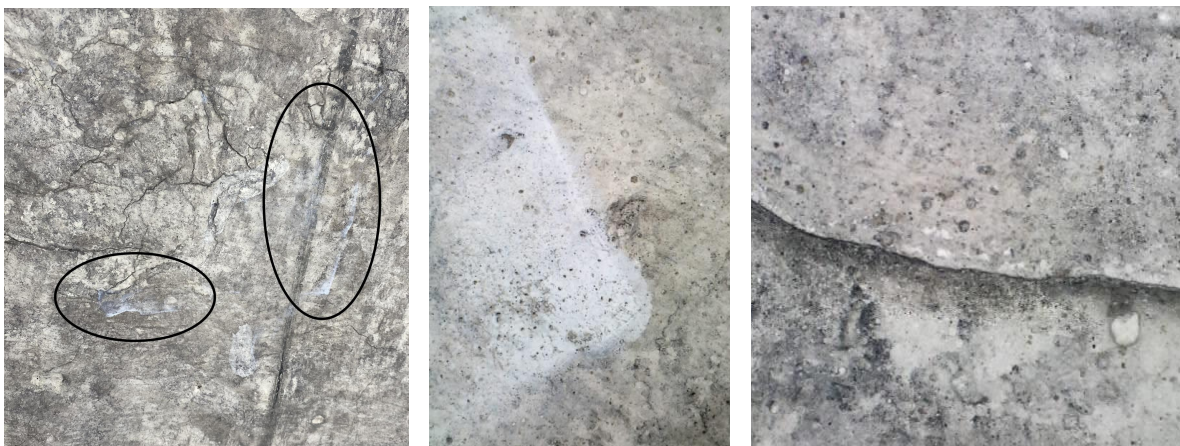
Figure 66 (left): Area B2: Formation of white haze after 1st application with Nanorestore Plus®
