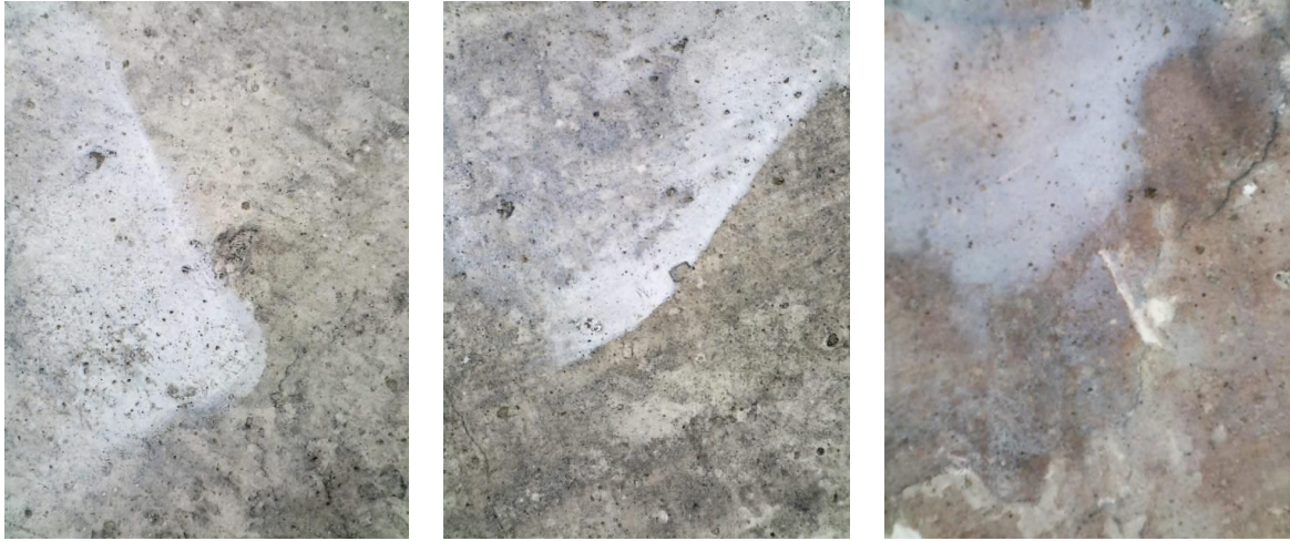
Figure 92 (left): Microscopic image, Area B2: formation of white haze after treatment with Nanorestore Plus®
