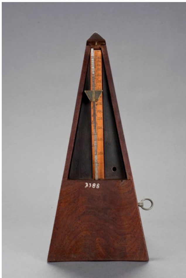
Figure 2. Maelzel metronome. The calibration of the scale goes from 50 to 160. The design of the scale clearly shows that the weight must be placed under the corresponding line. Musical Instrument Museum, Brussels, no. 3388.
