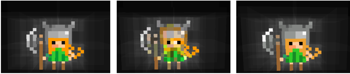
Figure 4.4: An example of how HSV can order colours to be closer to each other for the DXT1 compression results in better preserved quality when compared to an unsorted attempt. The image to the left is uncompressed, the middle is DXT1 compressed unsorted and the right image is DXT1 sorted using the permutation VSH, one of six possible permutation of HSV colour sorting. The model was derived from MagicaVoxel [32].
