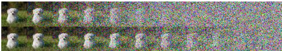
Figure 2.2: Forward diffusion process using linear (top) and cosine (bottom) noise schedules at evenly spaced intervals [11].
