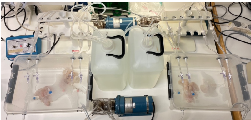
Figure 13. Picture of perfusion system including sheep uteri during decellularization
