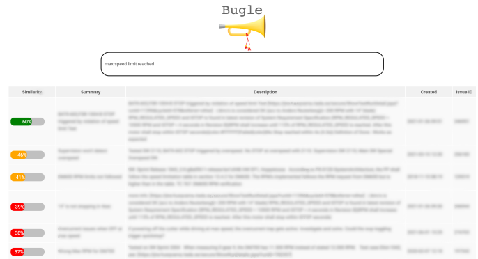
Fig. 4. Recommendations are displayed and ranked in a table as the user enters an issue description. Semantic similarity is normalized and color-coded in the first column to showcase the likelihood of a duplicate in the repository.
