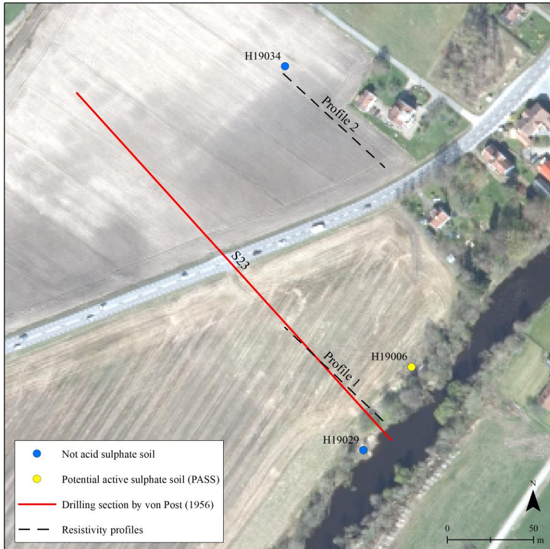
Figure 11. Top: Resistivity was measured along two 80-meter-long profiles. The profiles were placed next to the sample site H19006 (classified as potential AS soil) and von Post’s (1968) drill profile S23. The profiles were placed with 100-meter distance in order to overlap and cover as much as possible of S23. Bottom: the two measured resistivity profiles marked in von Post’s “Section 23”. The purpose was to see if it was possible to see one of von Posts interpolated sulfide layers or the sulfide layer found in this study with the help of geophysics. Orthophoto 4 band 0.16 m 2019 © Lantmäteriet. Drilling profiles by von Post (1968) digitalized by Elin Norström, SGU.
