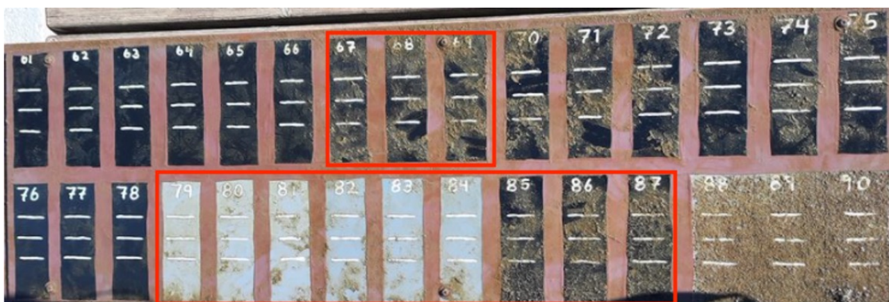
Figure 16: Full picture of panel retrieved from Girona site. Red boxes indicate the analysed paints in this study.
