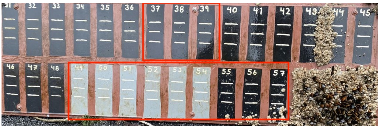
Figure 13: Full picture of panel retrieved from Gothenburg site. Red boxes indicate the analysed paints in this study.
