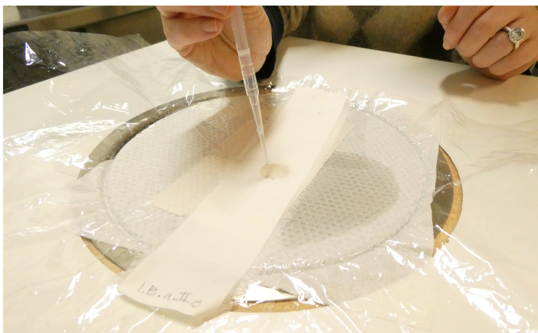
Fig. 12. Cleaning stained samples on a suction table. Photo by Johanna Nilsson.
