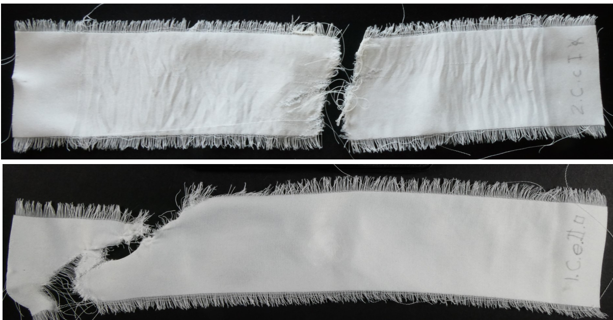
Fig. 52. The one sample that tore through the stain and one of the 66 samples that tore at the top of the sample.
