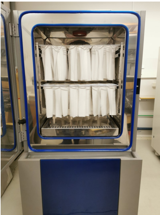
Fig. 9. The CTS climate chamber with all samples ready for ageing.
