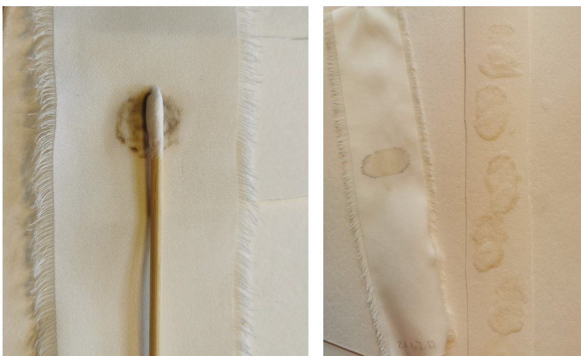
Fig. 11. Cleaning stained samples using cotton swabs and blotting paper.
