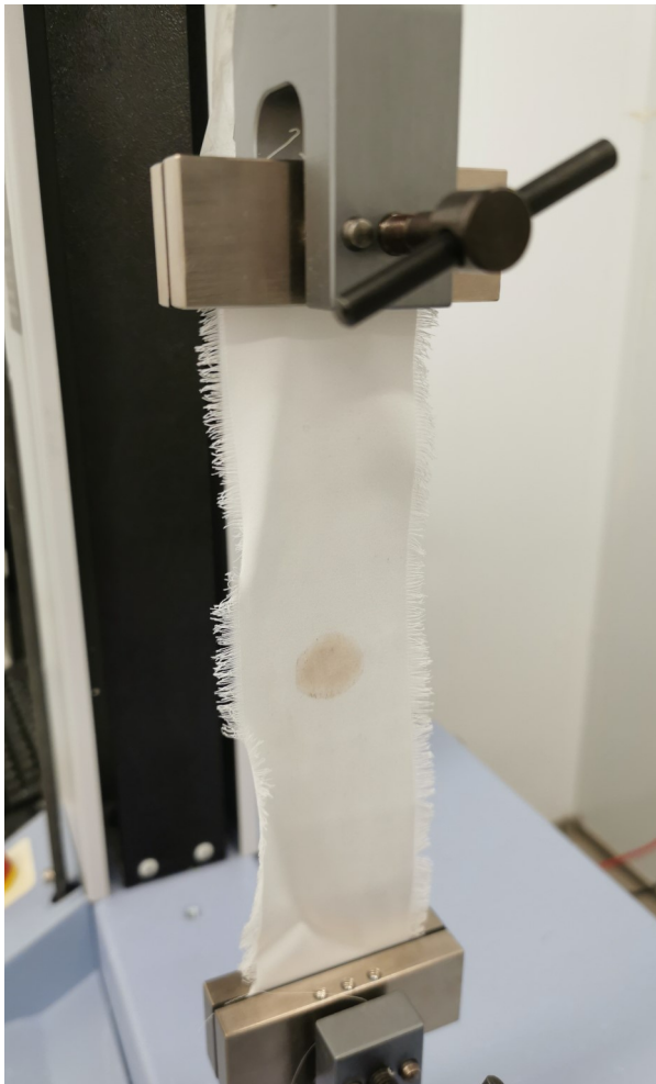
Fig. 13. Tensile testing of a sample stained with ashes.
