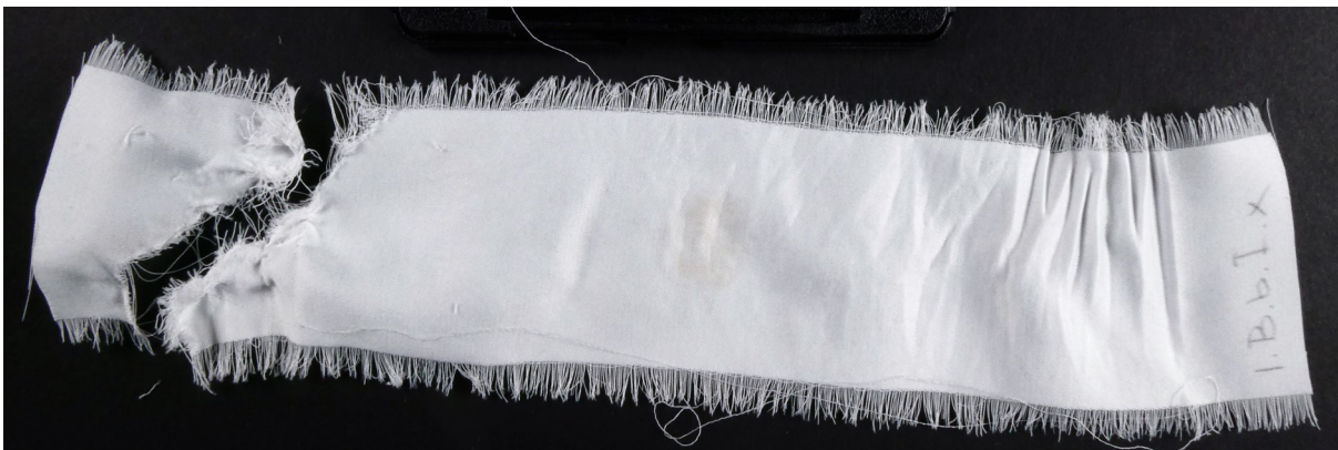
Fig. 48. Sample aged once and then stained with ash and cleaned with Dehypon. The tear from the tensile testing is situated at the top of the sample.
