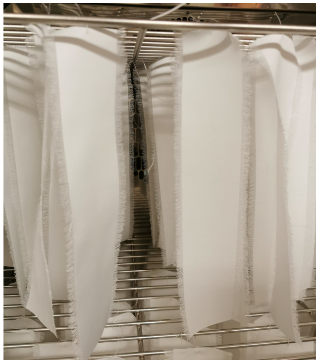
Fig. 6. Samples prepared with gauge length 200 mm and width 50 mm + fringe. The samples are placed in the climate chamber, ready for ageing.
