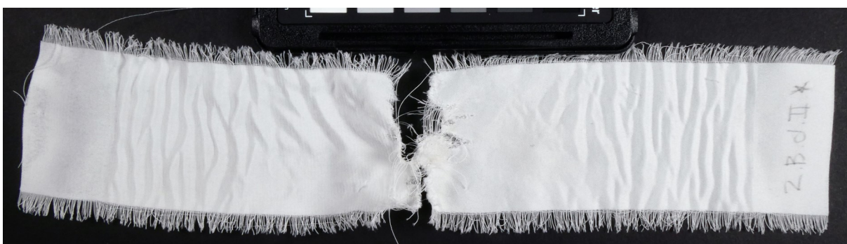
Fig. 49. One of the 18 samples torn straight through the stain. The sample is aged twice, and was stained with ash previous to and cleaned after the second ageing.
