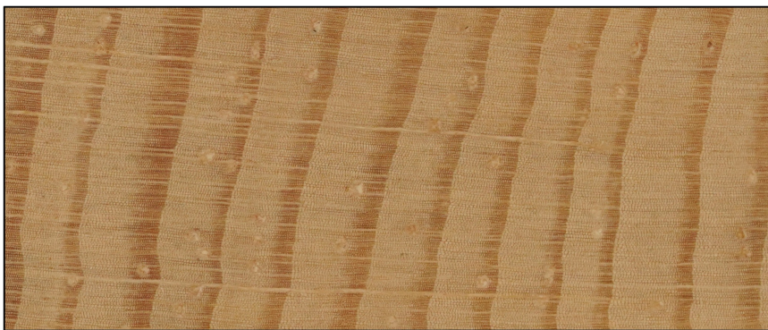
Figure 6. Sample GAP361 after being refluxed in 27 hours in 97% ethanol and sanded. Source: authors own.
