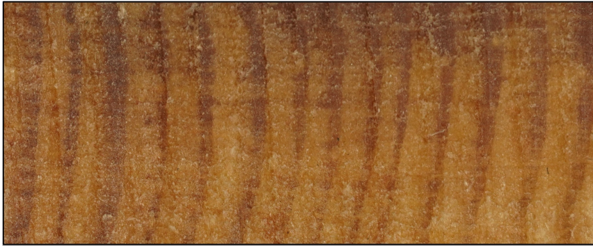
Figure 5. Sample GAP361 sawn from a disc of a dead Pinus Sylvestris L. with a high content of resin. Source: authors own.
