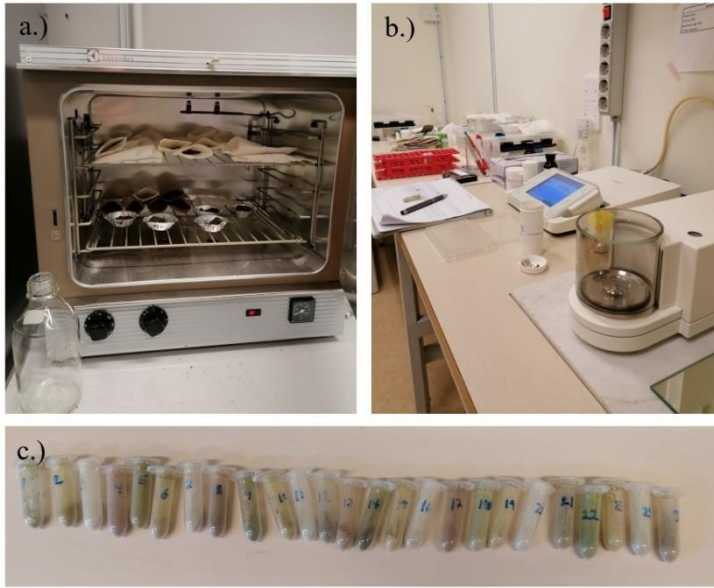
Figure 10. Pictures taken during the nitrogen analysis. Documenting the (a) samples drying in a drying oven and (b) preparation steps before the IRMS when the grounded samples are weighed and placed in tin capsules. Last image, (c) shows all the grinded samples displayed in a row.
