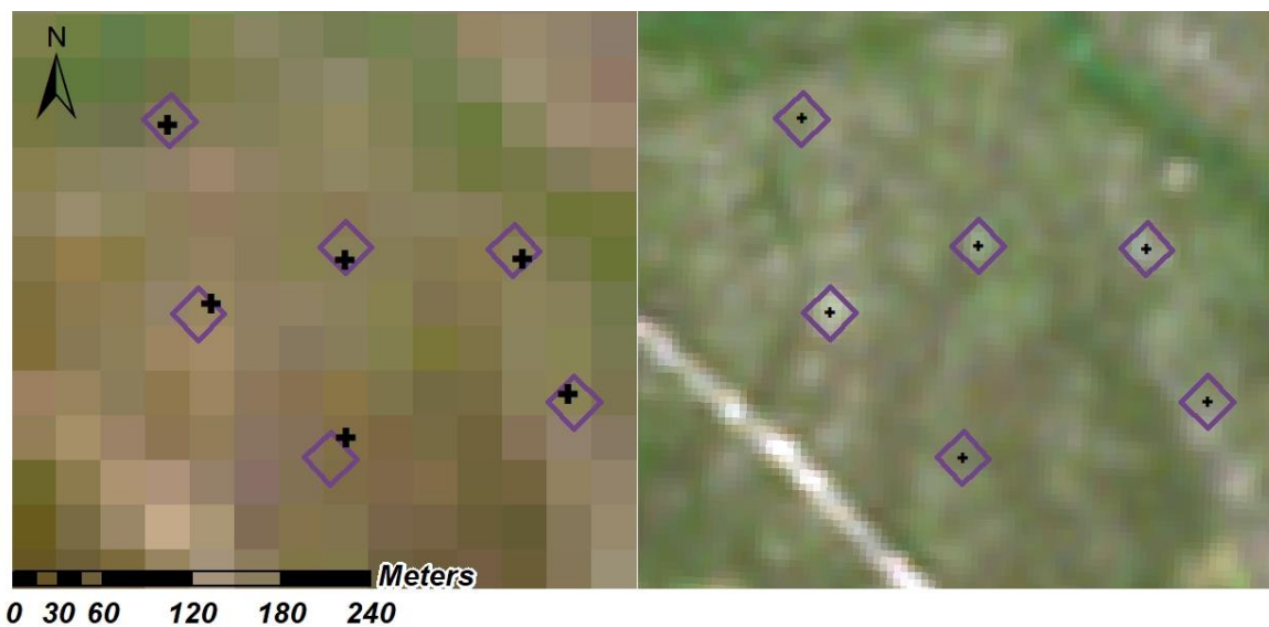
Figure 12. Displays which pixels were selected to represent the plots from the PRISMA (left) and Sentinel-2 data (right). For PRISMA the pixel with most area within the respective plots was selected to represent that plot. These cells are marked with black crosses in the map (left). For Sentinel-2 the centre pixels were selected, also shown as smaller black crosses in the map (right). The maps display ‘True color’ for PRISMA (30 m resolution) and Sentinel-2 (10 m resolution).
