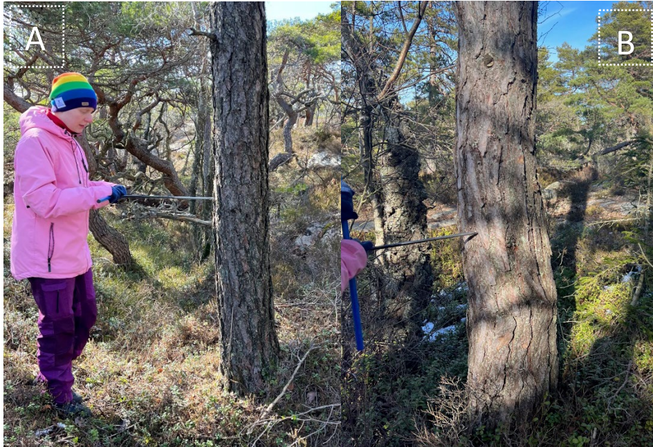
Figure 6. A) shows the angle when taking a tree sample from chest high. B) shows how the bore is aimed for the centre of the tree (pith).
