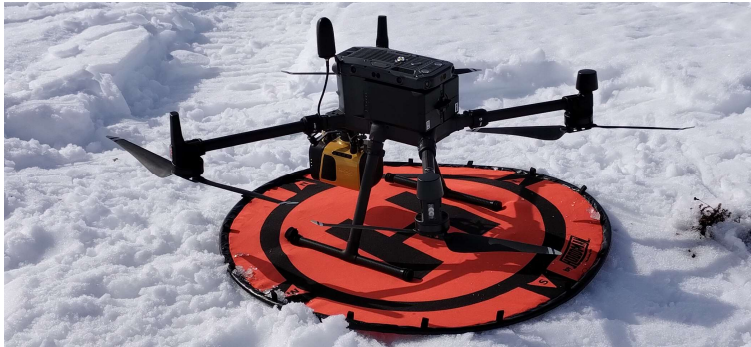
Figure 5. The DJI Matrice 300 drone carrying the YellowScan Mapper+ LiDAR scanner.
