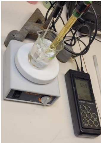
Figure 7. pH meter with both a pH and a temperature sensor.
