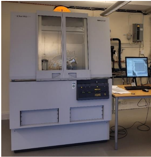
Figure 13a. The XRD instrument used in this study is at Naturhistoriska Museet in Stockholm, Sweden.
