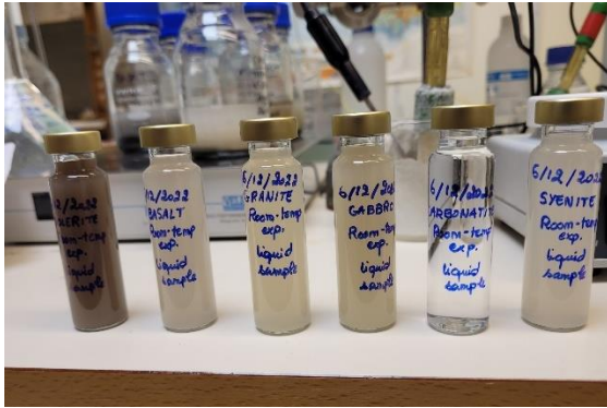
Figure 9. 20 ml liquid samples were extracted before further treatment with Na-rich solution.
