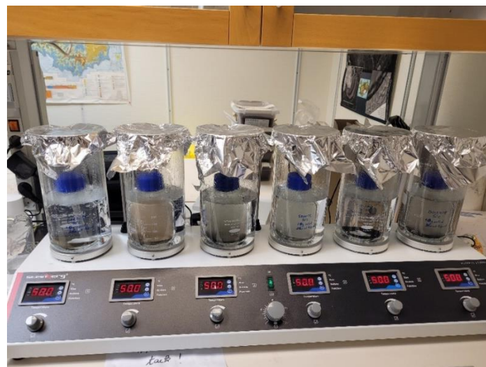
Figure 11. Set-up of the 50^{\circ}\text{C} experiments. Rock samples mixed with carbonated D.I water were placed in sealed glass bottles and placed in a 50^{\circ}\text{C} water bath which was then covered with aluminium foil to prevent water evaporation.
