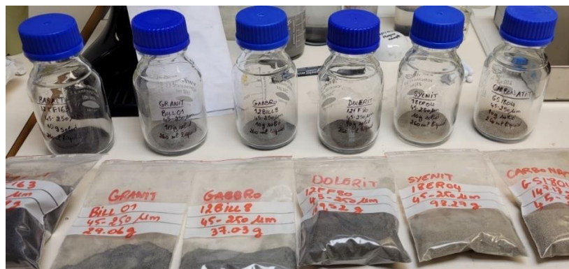
Figure 6. 10 g of the crushed rock samples are put in individual glass containers in preparation for experimentations.
