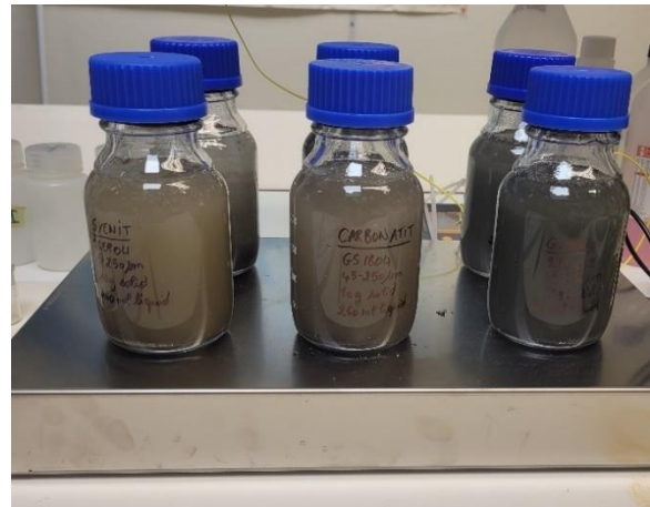
Figure 8. The containers including the rock samples and CO 2 D.I. water were placed on a magnetic stirring station for constant stirring during the room temperature experiments.
