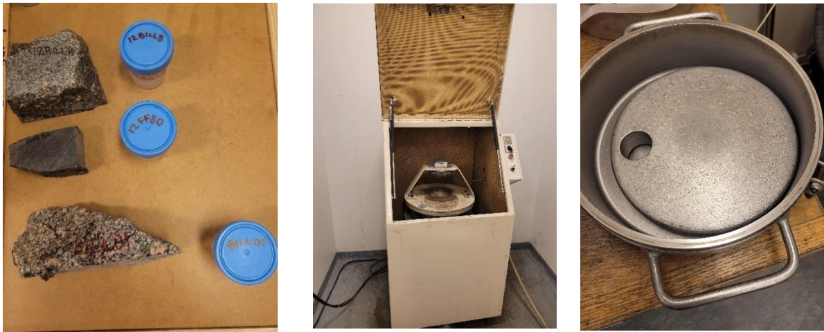
Figure 5. From left to right: 3 of the whole-rock samples used; the laboratory crusher; the metal container with the gyrating plate where the samples are put before being subjected to crushing.
