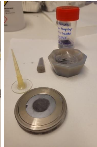
Figure 13c. : The rock samples mixed with acetone are manually ground to a fine powder and mounted on a pellet equipped with a zero diffraction plate.
