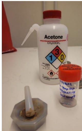
Figure 13b. Acetone was used to clean material and create a liquid solution using rock samples in an agate mortar.
