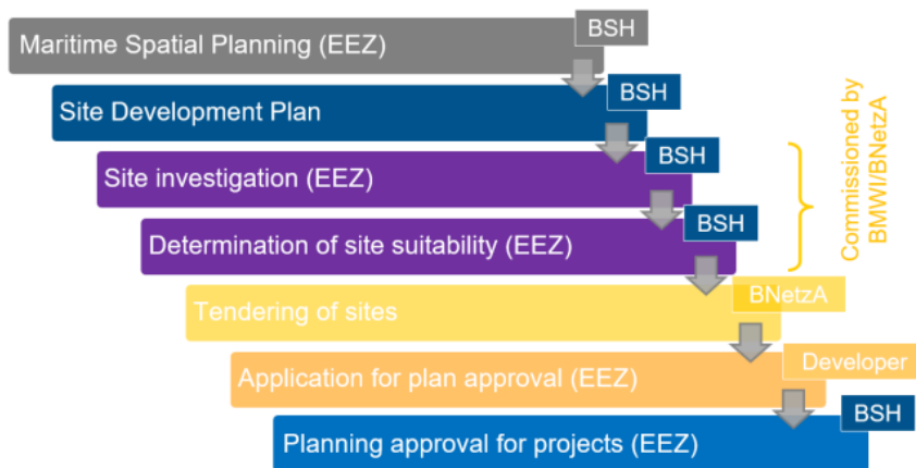
Figure 3. Central model of offshore wind energy planning (BSH, 2021).
